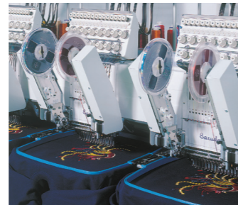
■ Double Sequin Device ● 双侧单珠片装置
